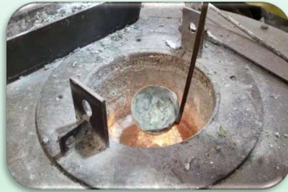
Magnesium alloy (AZ63B) melting under protective gas
