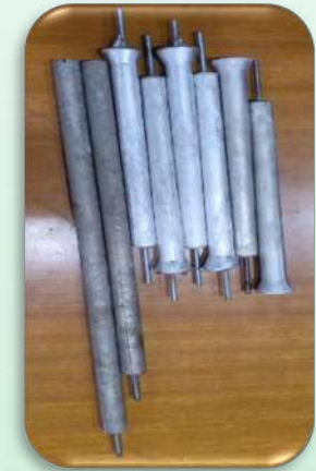
Finished magnesium anodes after fettling and inspection
