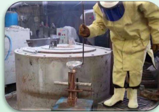
Controlled pouring of molten magnesium into mold
