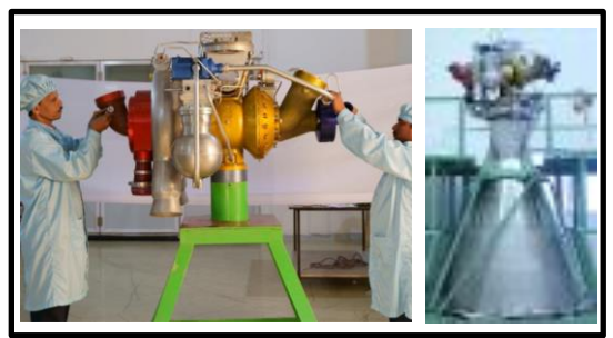
Liquid Propulsion Rocket Engine (Vikas Engine)
