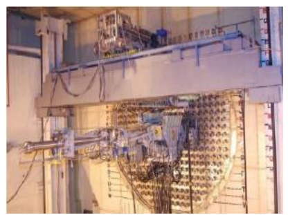
Fuel Machining Head operating in Nuclear Reactor
