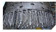
Control Plug for Reactor
