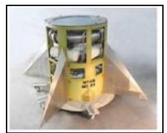
Base Shroud and Fin Assembly - Agni Programs: A1, A2, A3, A4, A5, A1 P
