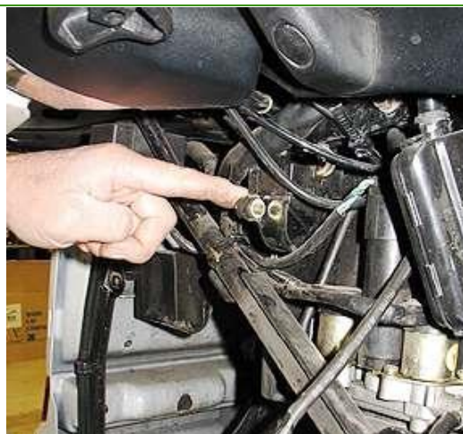
Exhibit 14: Positioning of Bank Angle Sensor in Bike
