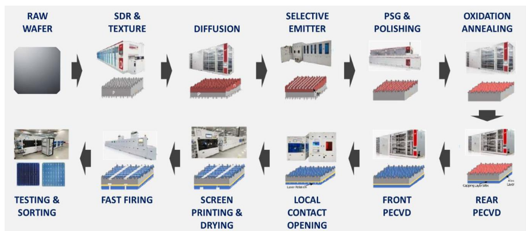
Exhibit 20: MonPERC solar cell manufacturing steps
