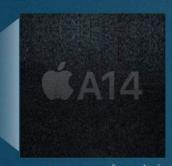
Processor chip: 88mm² size 8.57 mm x 10.23 mm
