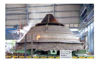
machining – both. Burden area of hopper & bell is hard faced with an alloy that doesn't require machining. Static balancing and leakage test is carried out to ensure 100% matching of seats. The performance life is enhanced considerably.
