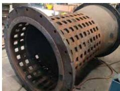
It used in Coal Washaries. When the gap becomes widens between rotor and outer body, the efficiency goes down. Screw, tiles and liners wear out due to abrasiveness of coal. The gap between rotor blades & body increases making it difficult to control feed rate and smooth operation of rotor.
