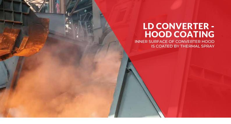
Converter Hood is a construction of number of tubes assembled together. Chilled water is circulated through these tubes to cool the hood. Tubes get thinned and then punctured due to severe abrasion at elevated temperatures caused by high velocity, airborne particles resulting into leakage in tubes and forcing a shutdown. Water if comes into contact with liquid metal, explodes and cause damage to human life as well as equipment.
