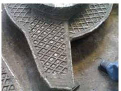
Both Sinter Crusher Star and Grizzly Bars are subjected to severe abrasion at very high temperatures.
