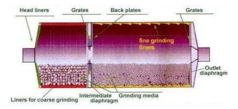
Tube mill use for grinding of raw material to the fine powder. Liners use for moments of grinding media. The diaphragm is work as a gate for transfer of raw material in and out to and from tube mill.
