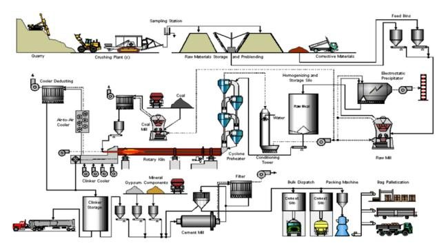
A process from limestone quarry to final cement manufacturing, we show it in details.
